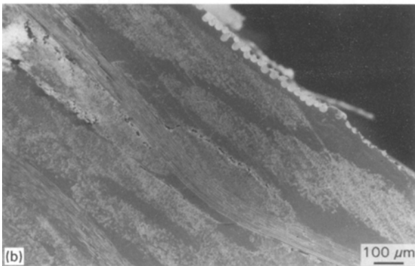
Figure 15 (a) Optical micrographs showing cracks around fibre bundles in a multiaxial (non-crimp) fabric hand lay up polyester at different impact energy levels and (b) SEM micrograph of fractures around a bundle in a glass reinforced epoxy eight-harness satin weave.
