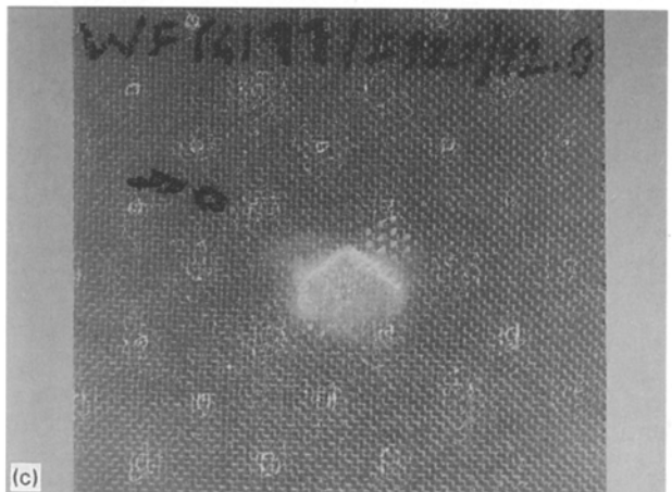
Figure 13 Impact damage in an eight-harness satin weave, glass fibre epoxy composite (a) SEM micrograph of cross-section through damaged region, (b) photograph of reverse (tensile) surface of impacted specimen and (c) photograph of contact surface of specimen.
